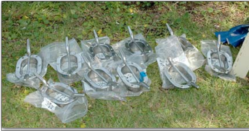
Hawse cleats – each one is custom-fit to its location on the boat
