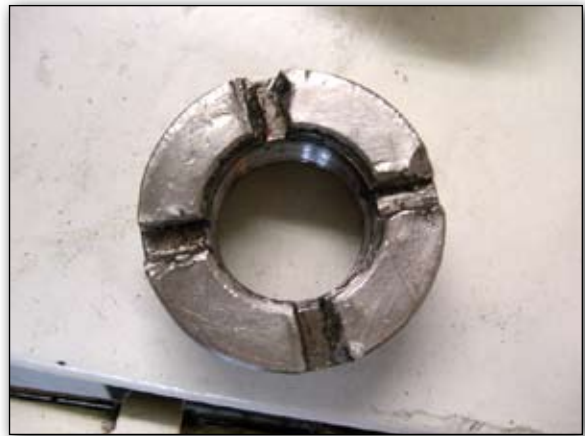
Drive Shaft coupling that backed off
