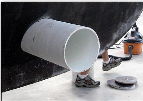
helm. Every other company wanted to do the whole installation, adding greatly to the cost of the project... about \$5K! We selected the "Binford" model, SE 170/250TC, an electric DC model with twin five blade counter-rotating composite props, a 10" tunnel and over 10HP that will thrust full on for over 30 seconds if necessary... arrrrgh!
